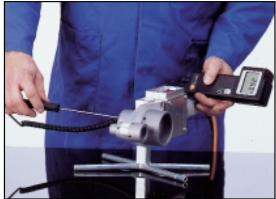
Temperature control by means of profile meter
