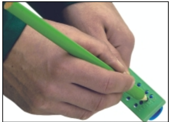
Marking the welding depth
